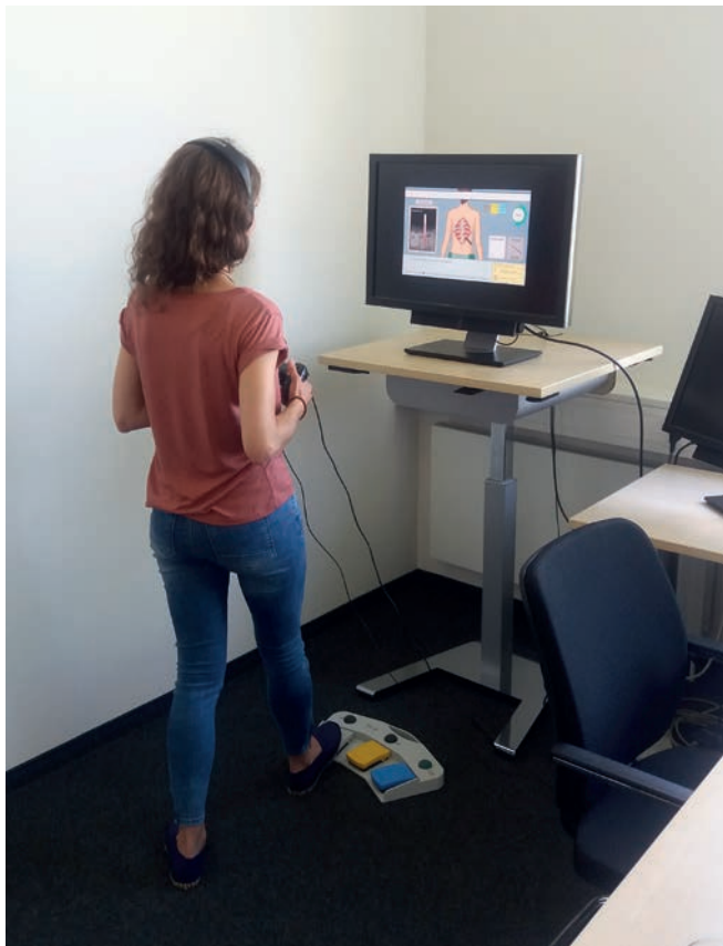
(Fig. 2). In collaboration with CITEC, steute tested different control concepts within the context of a spine operation. The photo shows the foot control prototype. A "division of tasks" combining foot and voice control proved to be the best solution.
