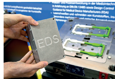
2K tools with an embedded system for diagnostics made by university of Schmalkalden, Moulding Expo 2015
